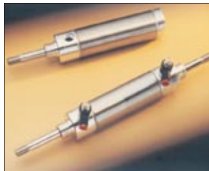
Fig. 5. Non-repairable cylinders generally are constructed primarily of stainless steel, aluminum alloys, and engineered plastics for pneumatic or low-pressure hydraulic service. Shown here are a single-acting, spring-return model, top, and double-acting with double rod-end, bottom.
