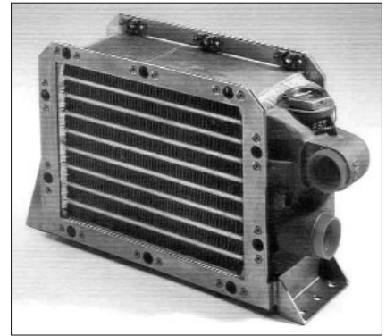
Fig. 3. Often found on mobile applications, oil-to-air heat exchangers use surrounding air to receive excess heat. Specially designed fins promote turbulent air flow to improve heat transfer capability.
