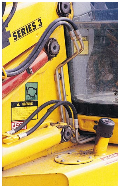
The interface between hose and rigid tubing is vulnerable to leakage caused by stress and strain induced by vibration, shock impulses, and differential expansion. To prevent leakage, hoses should be long enough to always remain slack, but be short enough to prevent rubbing against adjacent surfaces.
