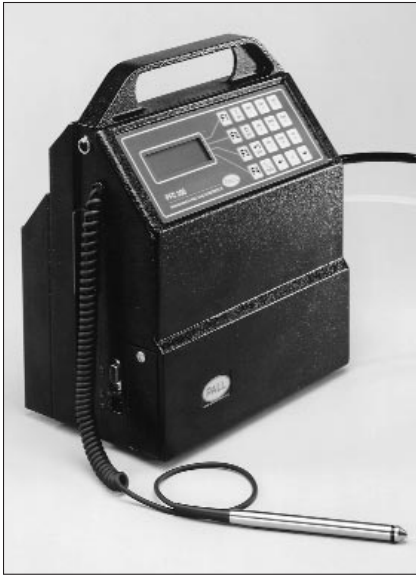
Fig. 1. Portable particle counter operates in three sampling modes: high pressure (from 50- to 5000-psi sources), low pressure (sources less than 50 psi), and from bottles. Typical analysis consists of three counting runs; instrument then displays cleanliness codes and average particle counts for seven micron-size ranges, and can produce reports from its built-in printer.
