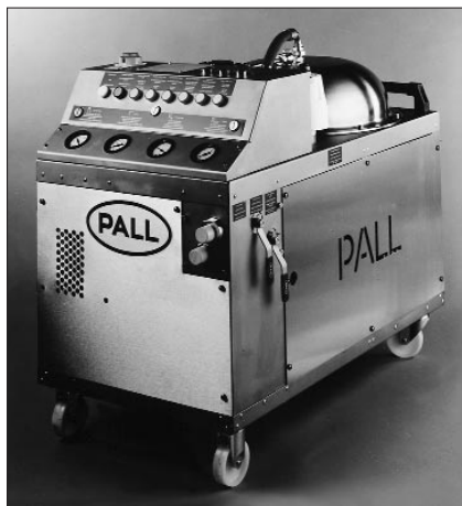
Fig. 3. Oil purifier removes free and dissolved water as well as free and dissolved gases. Nozzles spray water-contaminated fluid into its vacuum chamber; air with low relative-humidity passes through chamber to pick up water vapor and gases, then is discharged to atmosphere.
