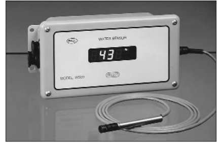
Fig. 2. Water sensor mounts in fluid line or hydraulic reservoir. LED display instantly indicates percentage of saturation and temperature, also flashes at 90% saturation to warn operator.
