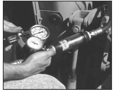
Fig. 6. Flow meters, unlike pressure gages, generally are not permanently installed in hydraulic or pneumatic equipment and must be piped temporarily in series with the circuit before use.
